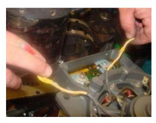
Figure 4—Field Coil Leads
