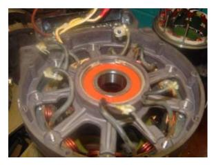
Figure 3—Phase Leads and Field Coil Leads
