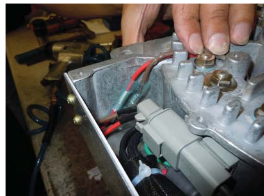
Figure 4 — Splicing to Field Coil Wires
