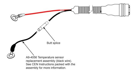
The entire temperature-voltage sense harness can also be replaced as an alternative to replacing just the sensor assembly. Contact your CEN Factory-Authorized Service Dealer or CEN Aftermarket Group for further information.
