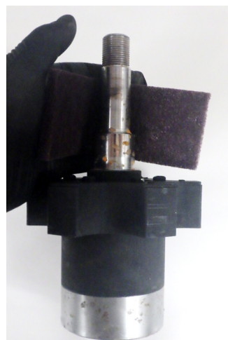
Figure 2: Remove Rust with Scouring Pad
