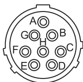
Figure 4 – Alternator-to-Regulator Harness Plug
