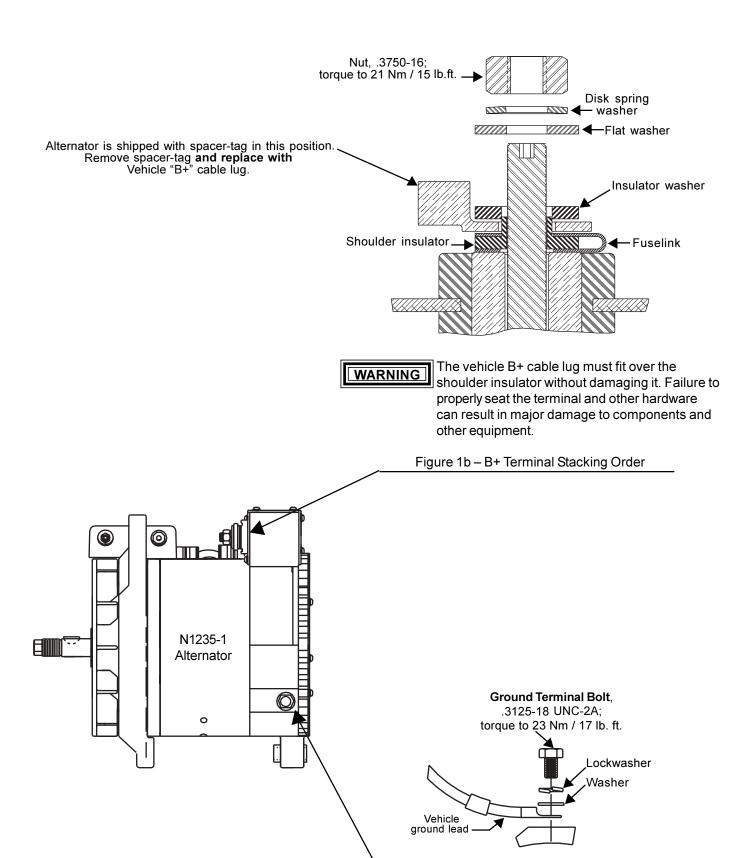
Figure 1c – Ground Terminal Stacking Order
