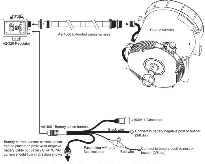
Figure 2 – Remote-Mounted A2-326 Regulator/C520 Alternator with Extended Wiring Harnesses
