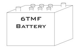
REGULATOR SETPOINT should be set to Position **#3** on underside of regulator for **6TMF** batteries installed IN ENGINE COMPARTMENT
