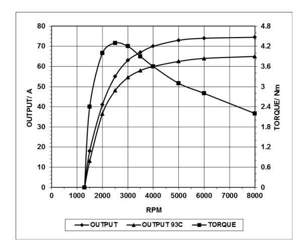
ALL MEASUREMENTS DEPICTED ON PERFORMANCE CURVES ARE TAKEN AT 104°F (40°C) AMBIENT TEMPERATURE (UNLESS OTHERWISE SPECIFIED) AND A STABILIZED MACHINE TEMPERATURE AT MAXIMUM OUTPUT CURRENT WITH VOLTAGE CONSTANT AS SPECIFIED PER SAE J56/ISO 8854.
