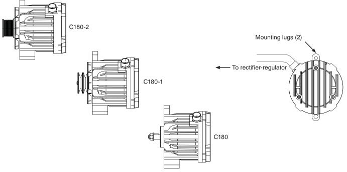
Figure 2 - C180-2/C180-1/C180 Alternator Details
