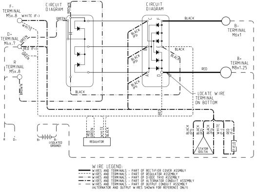
Figure 6 - C180-2/A2-207 Component Interconnection Diagram
