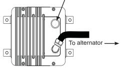
Figure 7 - A8-208 Rectifier-Regulator Cover Connections
