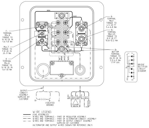
Figure 4 - C180-1/A8-206 Component Interconnect Diagram
