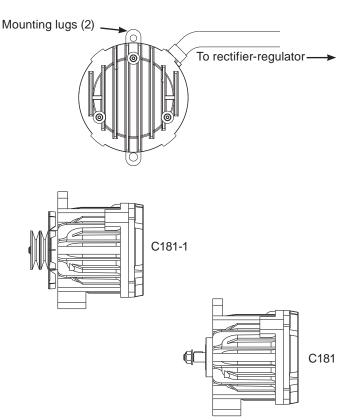
Figure 1 - C181-1/C181 Alternator Details
