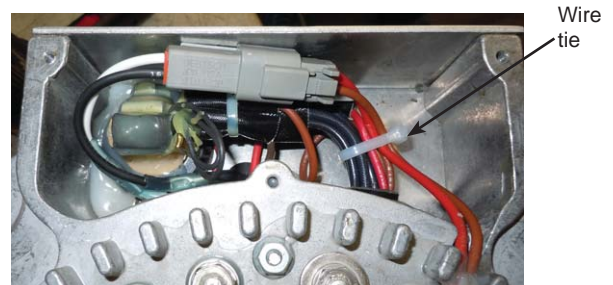
Figure 2 — Gray Field Connector Secured with Wire Ties Only
