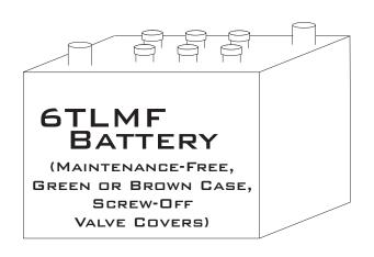
CEN N3264 Regulator Setpoint MUST be set to Position #2 on underside of regulator for 6TLFP or 6TLMF batteries
