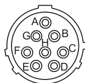
Figure 5 – Alternator-to-Regulator Harness Plug
