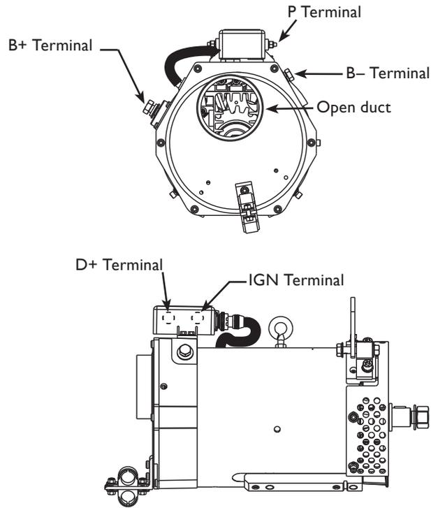
Figure 3 — C840D Alternator and A2-346 Regulator Terminals
