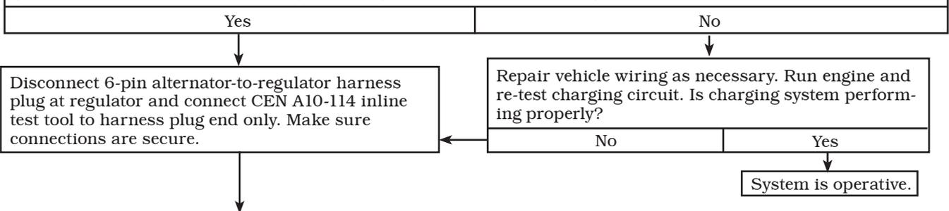
**MASTER BATTERY SWITCH ON, KEY OFF, ENGINE OFF:** Readings of all four tests must pass.
