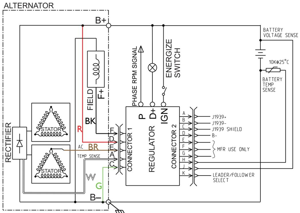
Figure 4 — C840D Alternator Schematic Diagram
